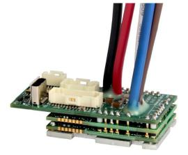
The **FM060-25-CM** is a single-axis servo drive and integration board assembly for a FE060-25-CM FlexPro<sup>®</sup> series servo drive with IMPACT<sup>™</sup> architecture. Connections to the controller, motor, power, and feedback are simplified through the standard connectors featured on the board.
