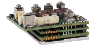
The **FM100-50-CM** is a single-axis servo drive and integration board assembly for a FE100-50-CM FlexPro<sup>®</sup> series servo drive with IMPACT<sup>™</sup> architecture. Connections to the controller, motor, power, and feedback are simplified through the standard connectors featured on the board.
