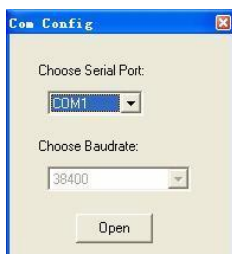
Figure 11: RS232 communication configuration window
