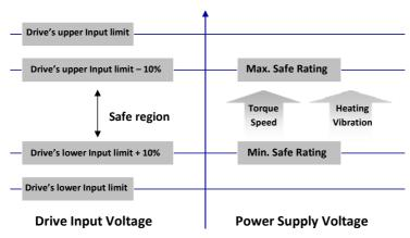
The recommended power supply voltage for DM805-AI is 24-72VDC:
