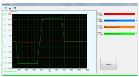
4. If Pr0.03 is set too small, it can cause the servo system to oscillate or become unstable, and the noise of the motor occurs, also alarm may appear. When Pr0.03=61, the operation of the motor becomes oscillatory.
